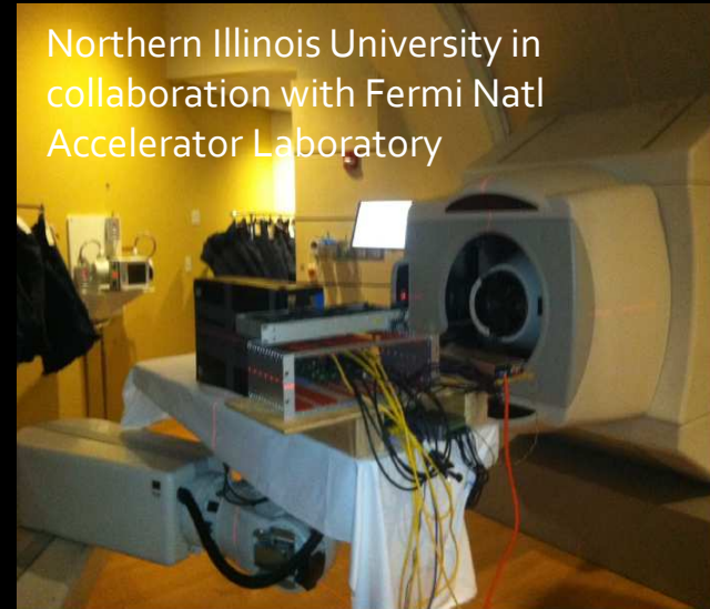
Figure 4.1: Test beam setup for range detector at ProCure Proton Therapy Center at Central DuPage Hospital.
